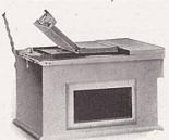
tor to properly place the negative and paper. When ready for exposure, the hinged pressure board is closed and locked, and a 60 Watt Mazda Lamp for which provision is made, is automatically lighted. The window on the side provides a safe dark-room light for developing out and bromide papers.
