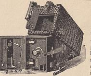
L ENSES of varying focal length may be used and the diaphragms changed without removing the shutter. A removable rear compartment is also made for use with the camera, which is fitted to contain five double holders and is adapted to take the place of the focusing cloth when the plate holders and rear partitions have been removed. This camera may be carried and operated in our patent satchel, thus giving it the appearance of an ordinary hand bag.
