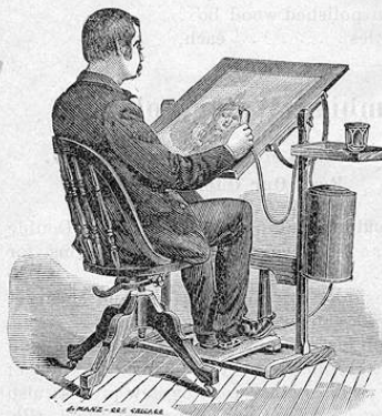
This cut shows manner of using the Air Brush.
