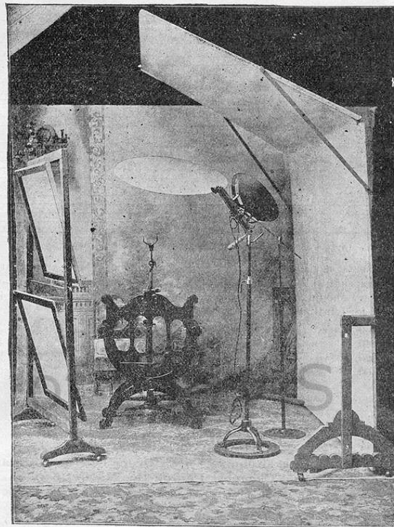
This design shows the position of Electric Lamp, Side and Head Screens.
